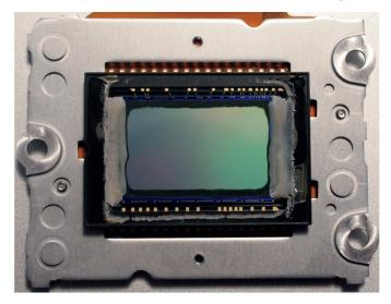
Figure 5 — Appearance of first successfully stripped D40 Sensor.
