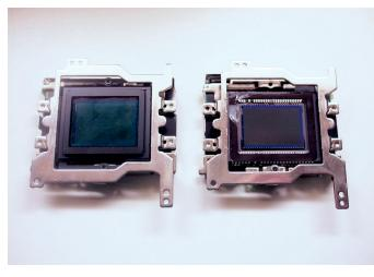
Figure 3 - Canon 10D CMOS sensors with ICF and AA filters, and without.
