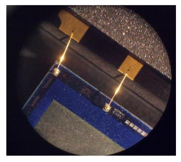
Figure 6 — Fragile gold connecting wires on D40 CCD sensor at  $100 \times$  magnification.
