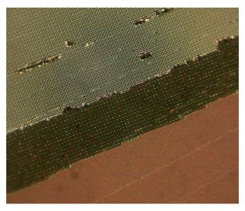
Figure  $4 - 100 \times$  magnification image of Nikon D40 sensor surface.
