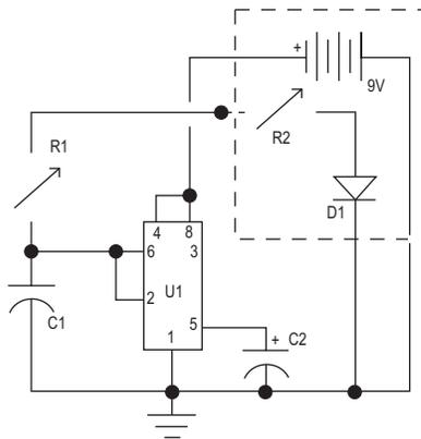
*Schematic diagram of the blinking reticle.*
